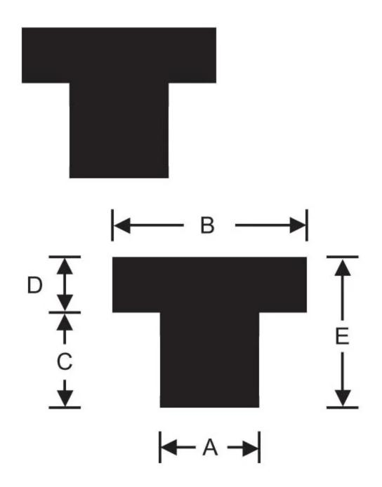
RPM's rubber recessed bumpers are used to protect doors or truck bodies from damage. They are also used as feet for large vibrating equipment.
