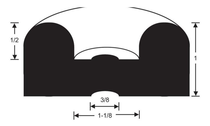
RPM's rubber recessed bumpers are used to protect doors or truck bodies from damage. They are also used as feet for large vibrating equipment.
