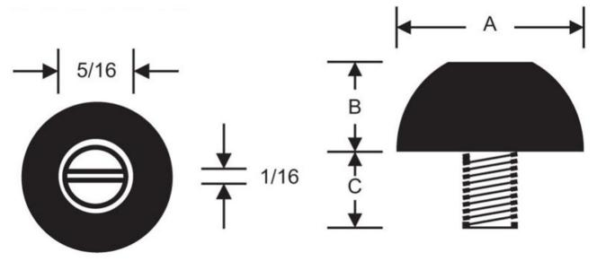
RPM's rubber recessed bumpers are used to protect doors or truck bodies from damage. They are also used as feet for large vibrating equipment.
