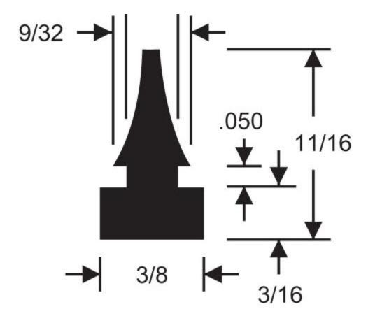
RPM's rubber recessed bumpers are used to protect doors or truck bodies from damage. They are also used as feet for large vibrating equipment.
