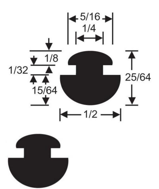
RPM's rubber recessed bumpers are used to protect doors or truck bodies from damage. They are also used as feet for large vibrating equipment.
