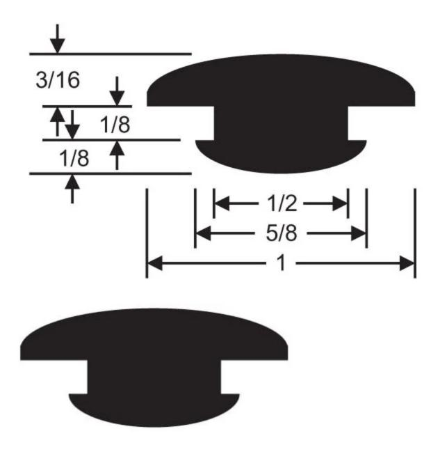
RPM's rubber recessed bumpers are used to protect doors or truck bodies from damage. They are also used as feet for large vibrating equipment.
