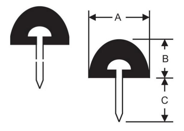
RPM's rubber recessed bumpers are used to protect doors or truck bodies from damage. They are also used as feet for large vibrating equipment.
