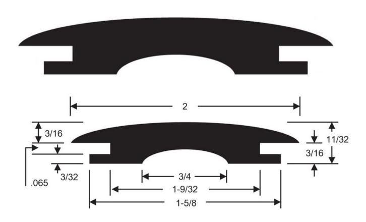
RPM Grommets are available in a variety of sizes to encompass almost any requirement.
