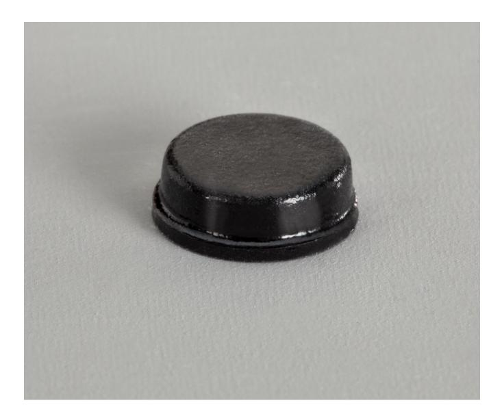
RPM Self Adhesive Bumpers are made of a permanently resilient polyurethane polymer formulated especially for its unique high coefficient of friction, non-slip, non-marring features. An aggressive synthetic rubber, high tack, pressure sensitive adhesive protected with an easy release liner makes application fast and easy.
