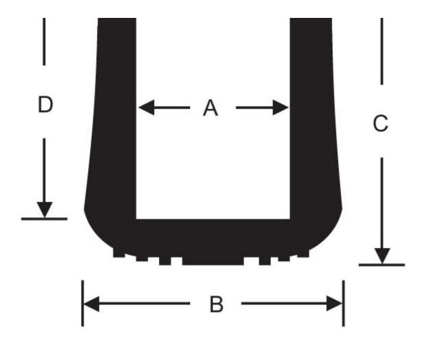
Standard types and sizes are available in black with durometer 60. Other colors and durometers are available by special order.
