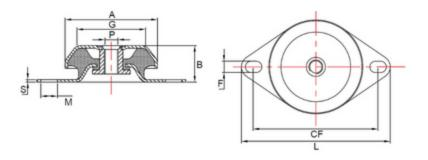
Flange mounts, or anti-vibration mounts, are universal mounting and popular in a wide range of applications and industries. Flange mounts are cost-effective, high-performing, and easy to install. The rubber is used in shear compression providing optimum performance and a wide range of flexibility. Offering vibration reduction up to 95%.
