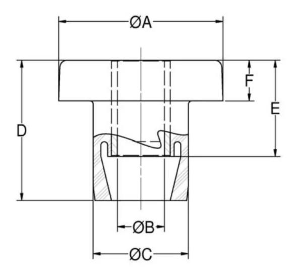
Center Bonded Mounts isolate vibration, control shock and reduce noise due to structure borne vibrations.
