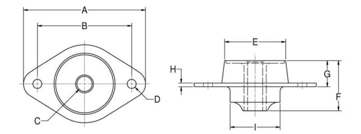
Center Bonded Mounts isolate vibration, control shock and reduce noise due to structure borne vibrations.
