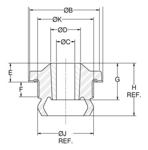
Center Bonded Mounts isolate vibration, control shock and reduce noise due to structure borne vibrations. Available in a full range of rated load capacities and able to withstand shock loads of 10 g's, these mounts effectively protect equipment and improve operator comfort. They are ideal for automotive, marine, railroad and industrial markets.
