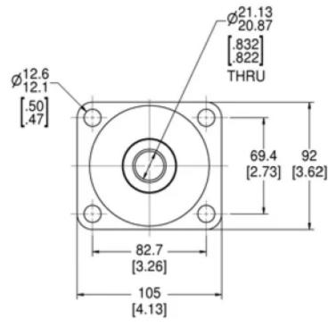
Conical mounts from Lord Corporation provide effective vibration isolation and noise attenuation with a simple, robust mount design. Consistent performance, high load bearing capabilities and a choice of radial stiffness characteristics are key features of these mounts. For more demanding vibration and noise reduction requirements, Lord integrates conical mounts with surface-effect technology to form an advanced control solution known as Hystec<sup>TM</sup> Systems.
