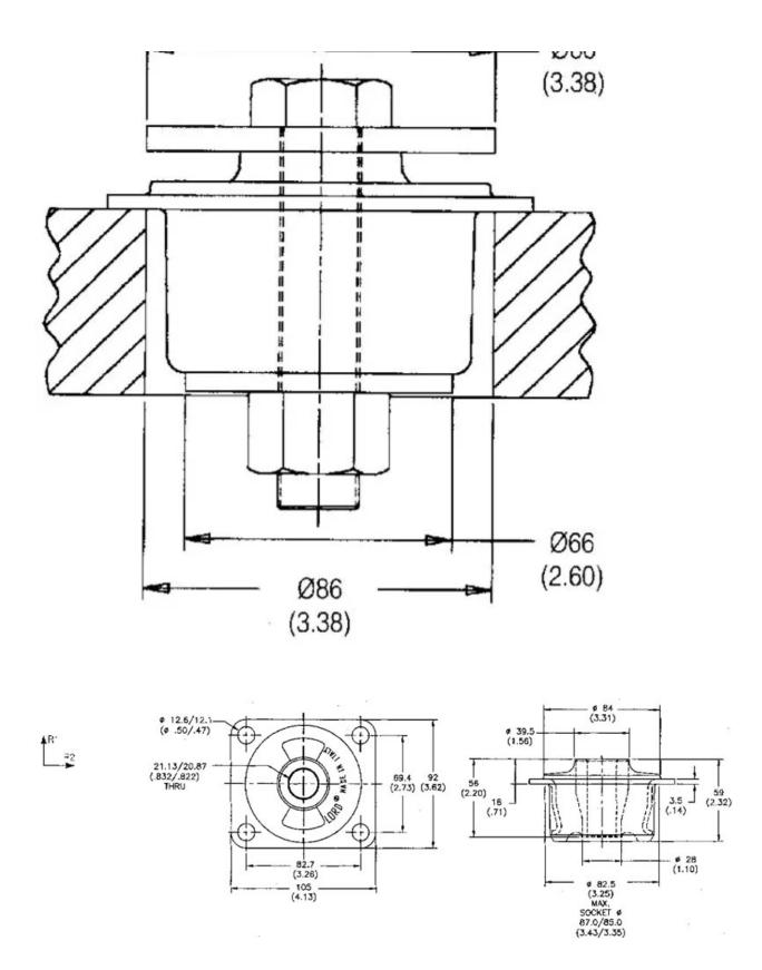
Conical mounts from Lord Corporation provide effective vibration isolation and noise attenuation with a simple, robust mount design. Consistent performance, high load bearing capabilities and a choice of radial stiffness characteristics are key features of these mounts. For more demanding vibration and noise reduction requirements, Lord integrates conical mounts with surface-effect technology to form an advanced control solution known as Hystec<sup>™</sup> Systems.
