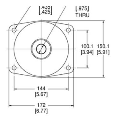
Conical mounts from Lord Corporation provide effective vibration isolation and noise attenuation with a simple, robust mount design. Consistent performance, high load bearing capabilities and a choice of radial stiffness characteristics are key features of these mounts. For more demanding vibration and noise reduction requirements, Lord integrates conical mounts with surface-effect technology to form an advanced control solution known as Hystec<sup>TM</sup> Systems.
