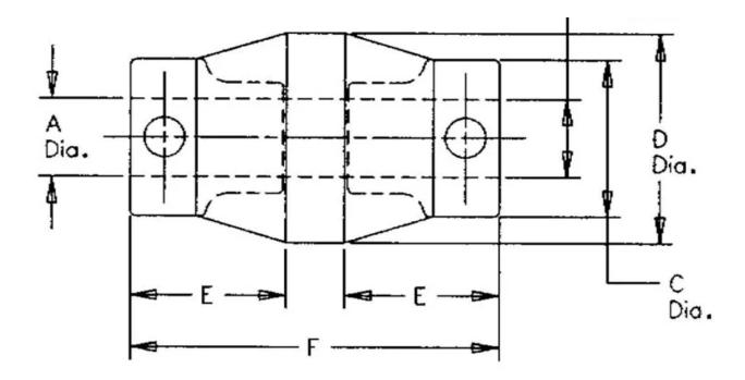
For Low Frequency Vibration Isolation and Misalignment Accommodation Compact, one-piece flexible couplings economically constructed to isolate low-frequency vibration and accommodate multi-directional misalignment.
