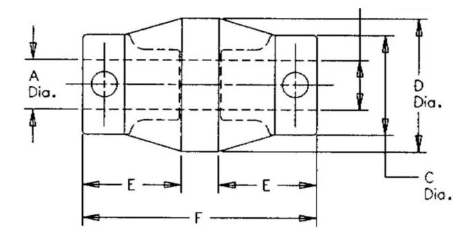
For Low Frequency Vibration Isolation and Misalignment Accommodation Compact, one-piece flexible couplings economically constructed to isolate low- frequency vibration and accommodate multi-directional misalignment.
