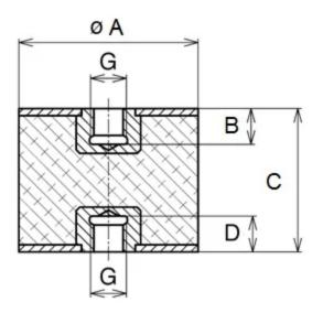
RPM Rubber Flex Sandwich Mounts are designed to protect equipment and machinery against damaging vibration. This family of mounts has excellent capacity for energy control.
