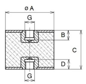
RPM Rubber Flex Sandwich Mounts are designed to protect equipment and machinery against damaging vibration. This family of mounts has excellent capacity for energy control.
