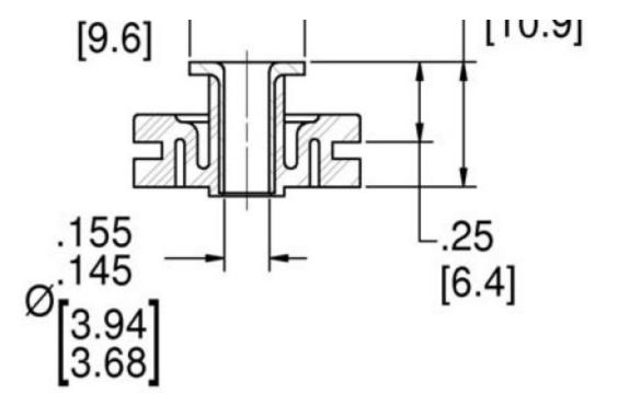
Lord Grommet Isolators provide effective, economical vibration isolation for light loads. They are suitable for commercial and military applications including computers, disk drives, business machines, precision instrumentation and general industrial equipment.
