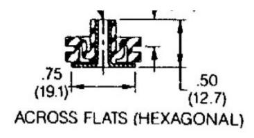
Lord Grommet Isolators provide effective, economical vibration isolation for light loads. They are suitable for commercial and military applications including computers, disk drives, business machines, precision instrumentation and general industrial equipment.
