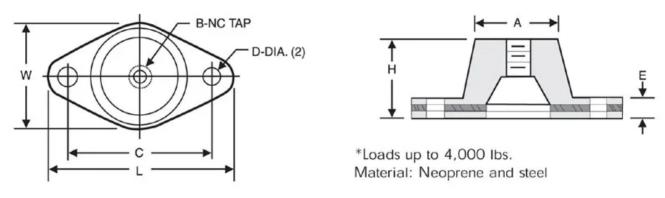
RPM's flange mounted compression mounts offer a quick and easy way to isolate your equipment. Simply fix the base of the mount to your surface and place your unit on the top surface of the RPM's Double Deflection mount series ensure your equipment keeps running and operating efficiently.
