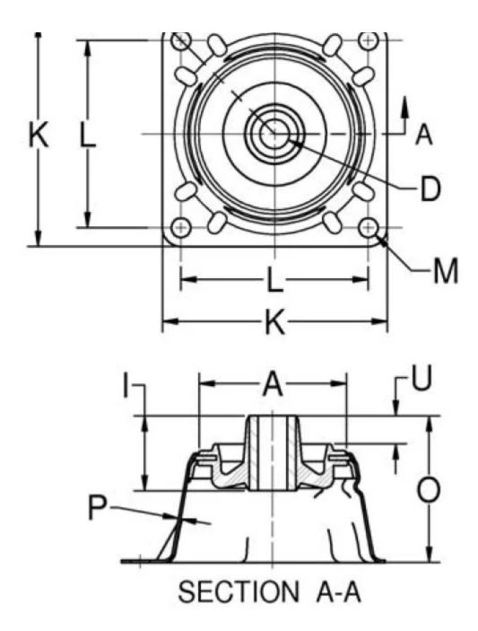
Lord Plateform Mounts provide effective isolation against vibration. The contour of the flexing element was developed to provide uniform stress distribution. This, plus high strength bonding and the use of specially compounded elastomers, provides maximum service life.
