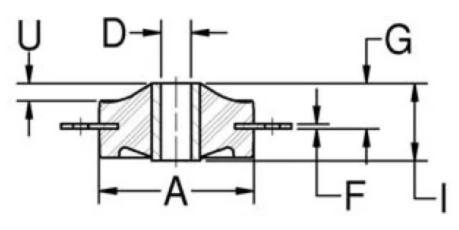
Lord Plateform Mounts provide effective isolation against vibration. The contour of the flexing element was developed to provide uniform stress distribution. This, plus high strength bonding and the use of specially compounded elastomers, provides maximum service life. Snubbing washers provide an interlocking system of metal parts which act to prevent damage from overload or excessive shock impact.
