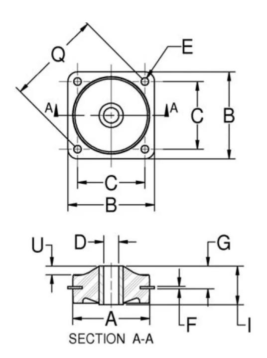
These versatile mounts are available in three types, each type featuring square, diamond or holder configurations to suit a variety of design requirements. The three types, Plateform Mounts, Heavy-Duty Plateform Mounts and Multiplane Mounts, offer a range in load ratings from 0.5 to 600 pounds.
