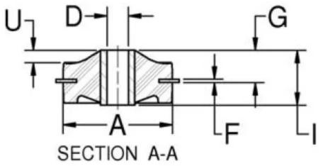
These versatile mounts are available in three types, each type featuring square, diamond or holder configurations to suit a variety of design requirements. The three types, Plateform Mounts, Heavy-Duty Plateform Mounts and Multiplane Mounts, offer a range in load ratings from 0.5 to 600 pounds.
