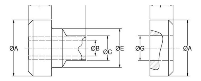
Two-Piece Mounts are designed for applications involving severe dynamic forces in the static load direction, as well as the rebound direction. Travel is limited in both directions by rubber in compression which provides snubbing.
