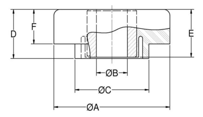
Two-Piece Mounts are designed for applications involving severe dynamic forces in the static load direction, as well as the rebound direction.
