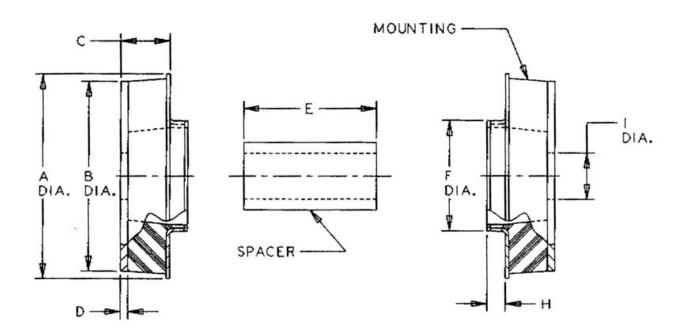
Two-Piece Mounts are designed for applications involving severe dynamic forces in the static load direction, as well as the rebound direction. Travel is limited in both directions by rubber in compression which provides snubbing.
